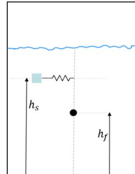
Figure 4. Sloshing model for a cylindrical tank
