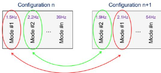
Figure 3. Mode shapes interpolation between different configurations
