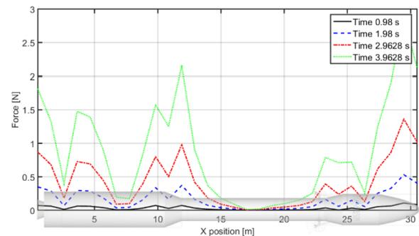
Figure 10. Local aerodynamic forces along the length of the launcher structure and function of the simulation time.
