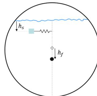
Figure 5. Sloshing model for a spherical tank
