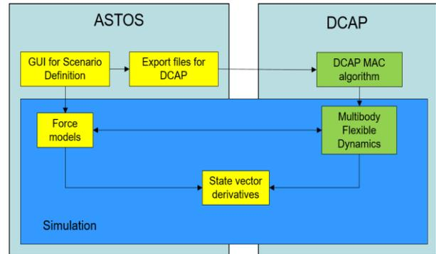
Figure 1. Interactions of DCAP and ASTOS in LauMBS software
