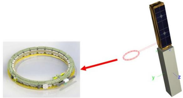
Figure 7. Clamp band device between the upper stage and the payload
