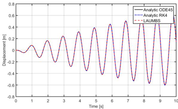
Figure 6. . Sloshing mass offset displacement for an external force acting on the tank with a frequency of 1 Hz
