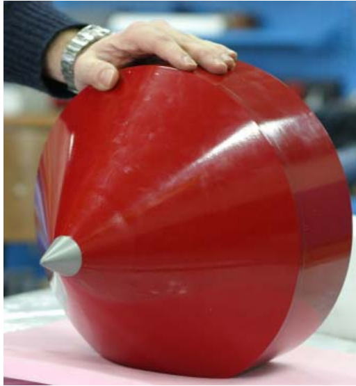
Figure 3 Fully integrated SHARK capsule.
