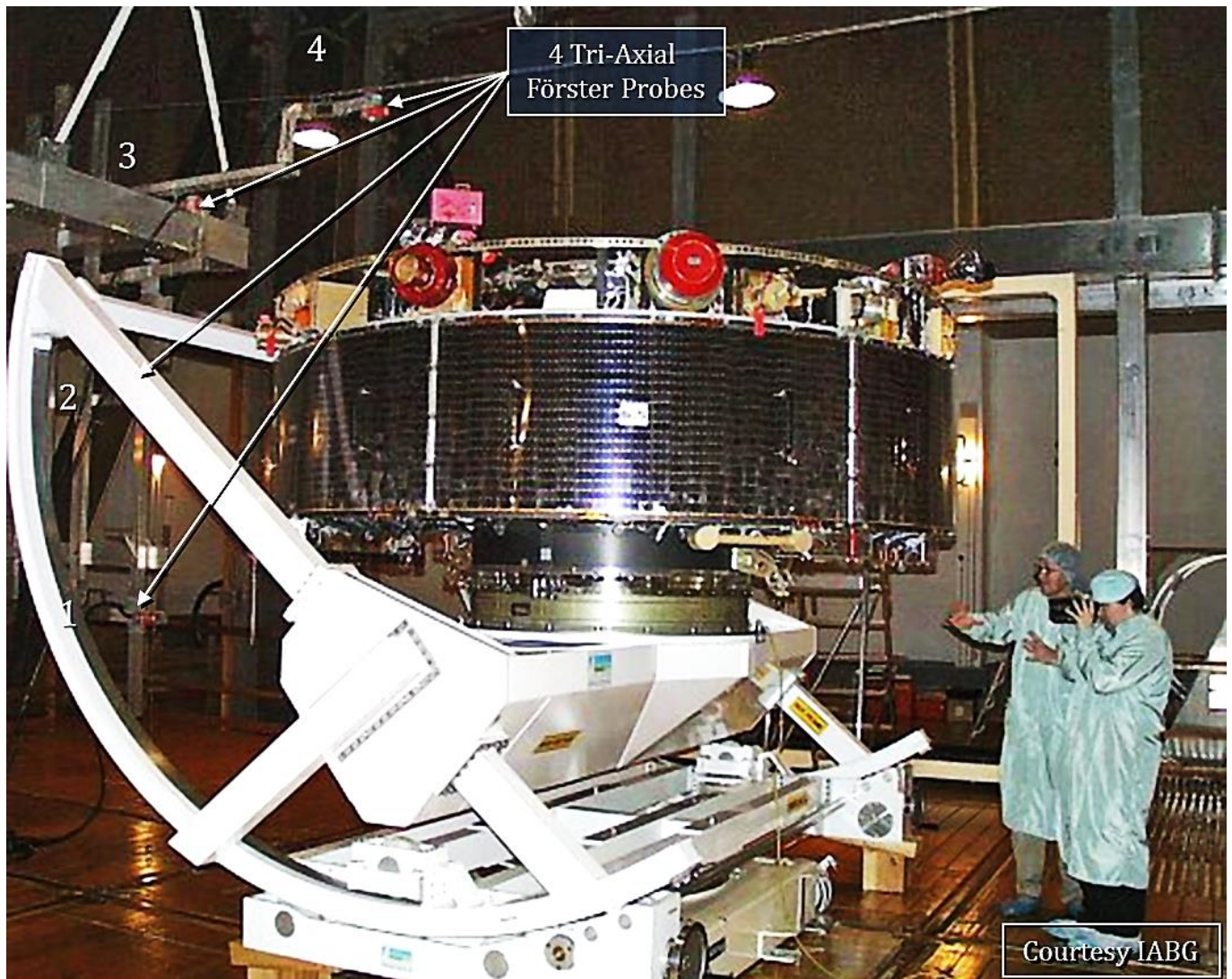
Fig.6 A Spacecraft in the Large Coil Facility of IABG, Munic, Germany
