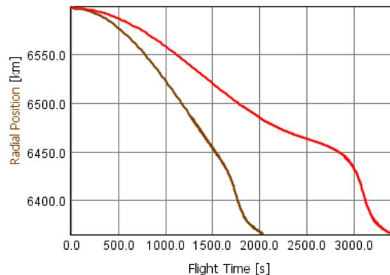
Figure 14. Radius evolution of two orbits with different perigee altitude (80 km in red, 0 km in brown)
