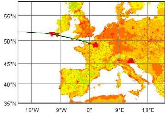
Figure 13. Impact footprint of two orbits with different perigee altitude (80 km in red, 0 km in brown)
