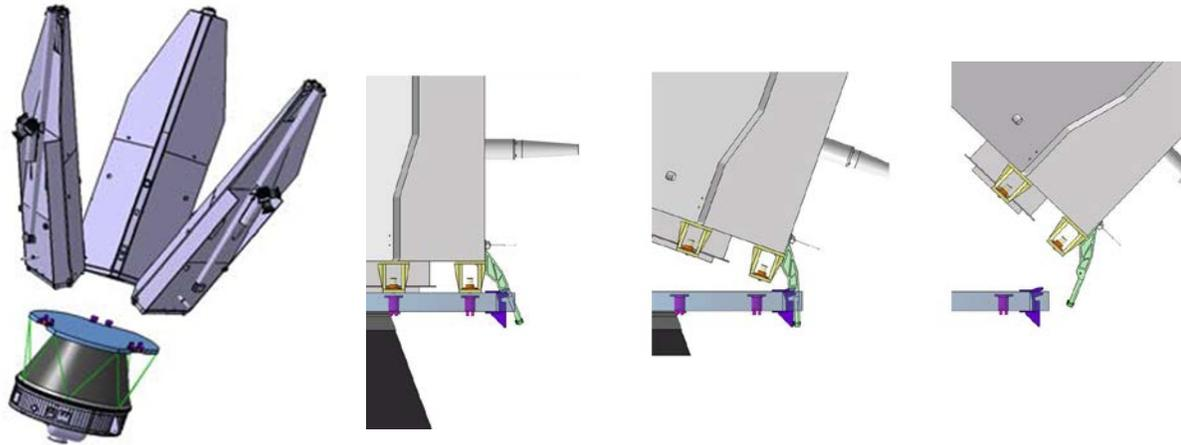
Fig. 6: SWARM satellites separation system
