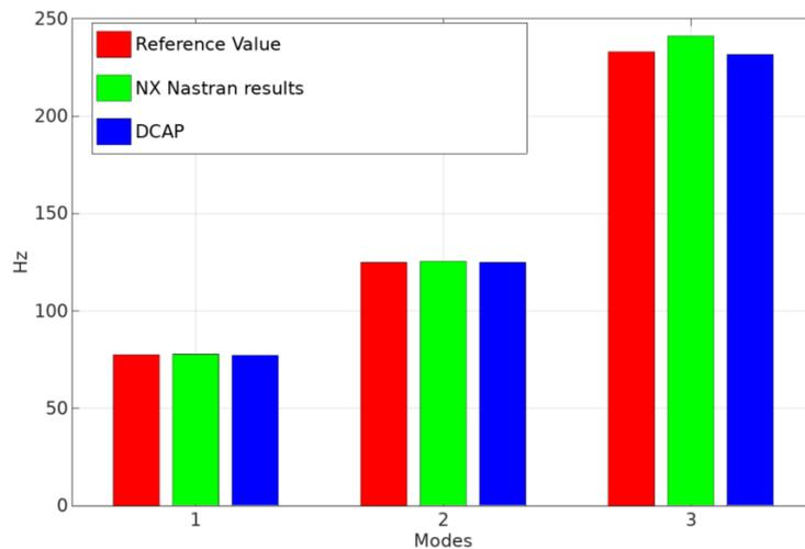
Fig. 13: Comparison of torsional and axial modes with benchmark analytical reference and NASTRA NX v10
