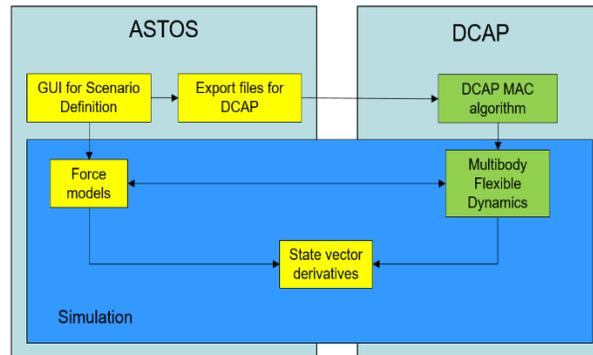
Fig. 14: DCAP and ASTOS interaction framework
