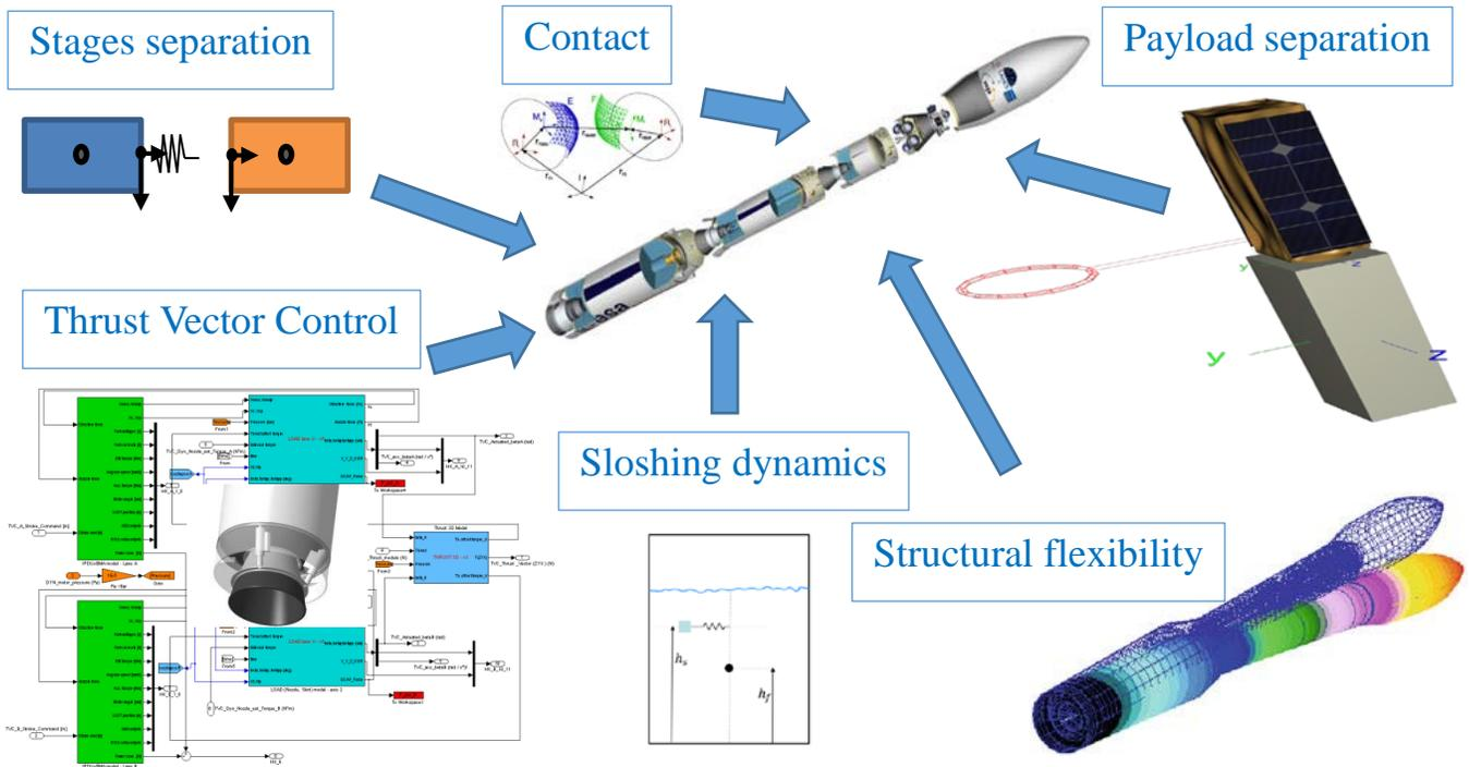
Fig. 2: DCAP launcher simulator features
