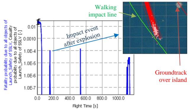
Fig. 3: Casualty and fatality probability during launcher ascent after explosion with increased probability during launch and close to islands.
